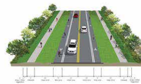
Typical Section #3 2-Lane Road with Sidewalks and Bike Lanes (Without Curb and Gutter)
