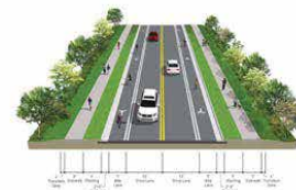
Typical Section #6 2-Lane Road with Sidewalks and Bike Lanes (With Curb and Gutter)
